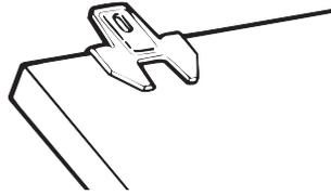
1. Edge Grip Clips are driven along both edges of the Durasan panels with attention not to over drive or allow points to move up towards vinyl surface.
