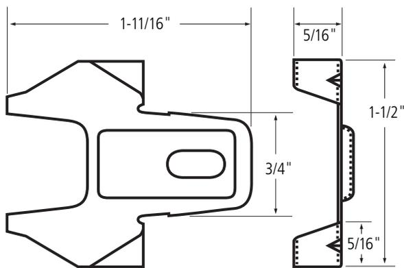
Edge grip clips provide for a simple one-step partition. The patented clips work with common framing wood or metal. Refer to pages 9 and 10 for installation recommendations.
