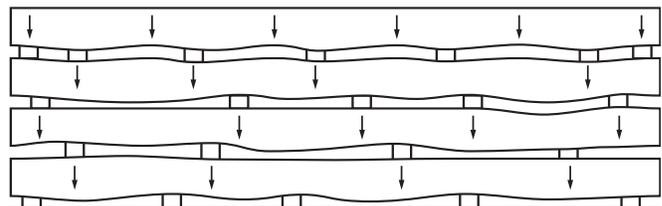
Cumulative pressure on unsupported lower units causes gypsum board to sag. Risers are not spaced evenly or in proper vertical alignment.
