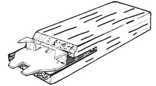
3. Using a hammer, tap the end of the installation tool until both teeth of the clip are fully inserted and the back legs are tight against the edge. Do not over drive the clips, as this can cause deformation of the board edge.
