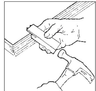
Apply clips to the leading edge of the panel 16" o.c., starting 16" down from the top. Clips on the trailing edge of the next panel are also spaced 16" o.c. but are about 2" from those on the first panel's leading edge. If greater rigidity is desired, clip spacing may be reduced. All panels require clips along both edges except when panels abut doors, windows, intersections or corners, in which case one edge of the panel will be directly fastened with nails or screws.
