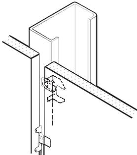
3. Clips on adjoining panel slide behind the first panel without screws.
