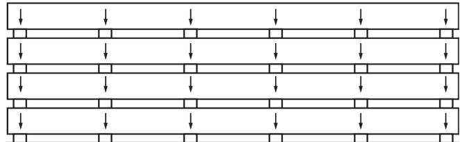
Note that all risers are placed in proper vertical alignment so each tier is evenly supported. Arrows indicate pressure.
