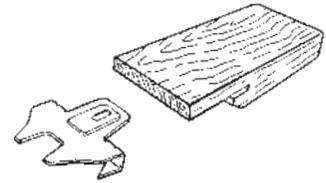
2. Position the clip and tool, as shown, against the back surface of the Durasan so that the clip is flat to the back, and perpendicular to the edge of the Durasan.
