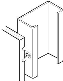
2. With edge of panel centered on stud face, clip is secured with standard Type S Pan Head Screws.
